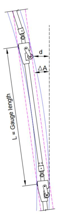
Below we list the range of allowed deformation in the inclinometer casing (consequently the borehole itself) that will give proper result while plotting the displacement profile.
